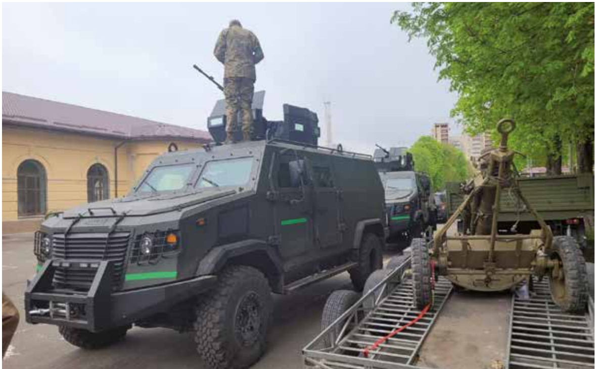
“Cossack” – A new locally produced armored vehicle based on the Ford F350 chassis.
